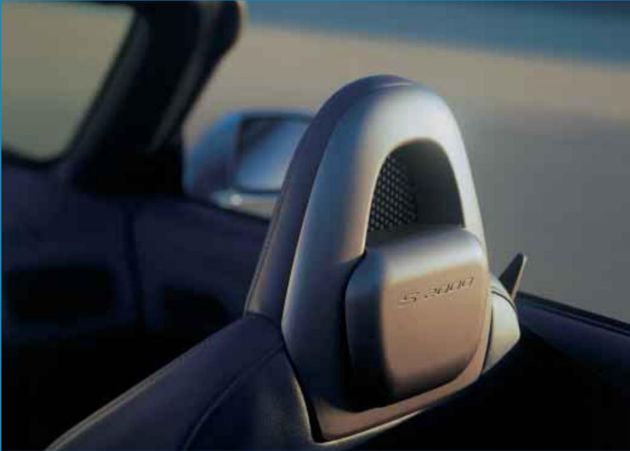
To further improve sound quality with the roof down, speakers can be compactly fitted into the rear of the headrests (also available for previous Honda S2000 models).
