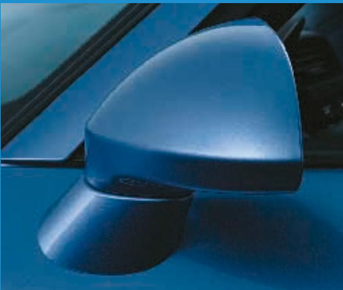
*You'll love to drive the Honda S2000 even when the sun's not shining, so the mirrors have heated elements behind the glass to ensure rear visibility.*
