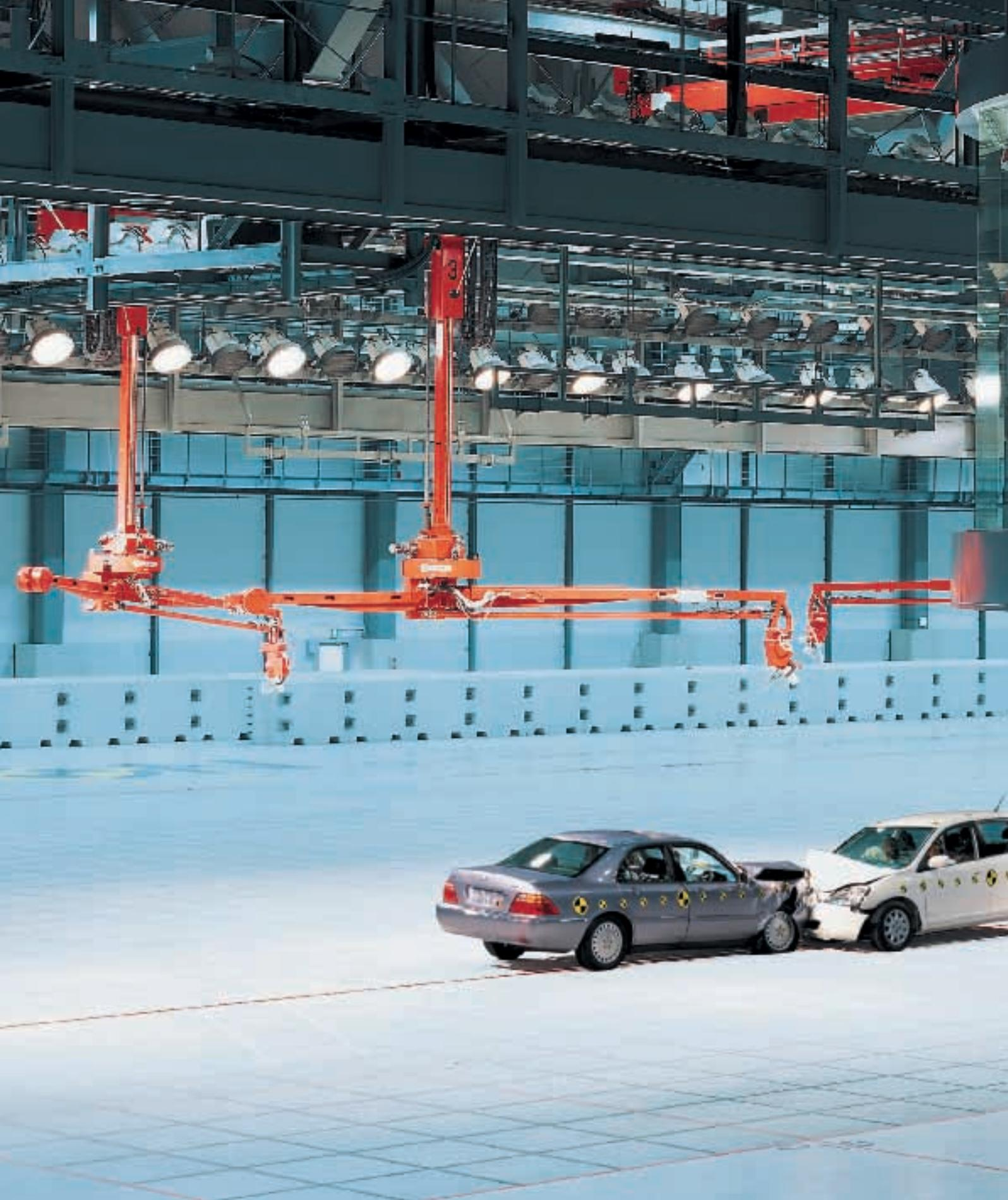
The Honda S2000 has been subjected to vigorous safety tests. We know just how hard a test regime the car's been through, as we built the test-facility centre ourselves. Our crash test centre in Tochigi, the largest in the world, has allowed us to test impact resilience from all possible directions, just as it can happen in real life. Within the car's frame are built-in crumple zones. These ensure that if an accident happens, the sections deform
